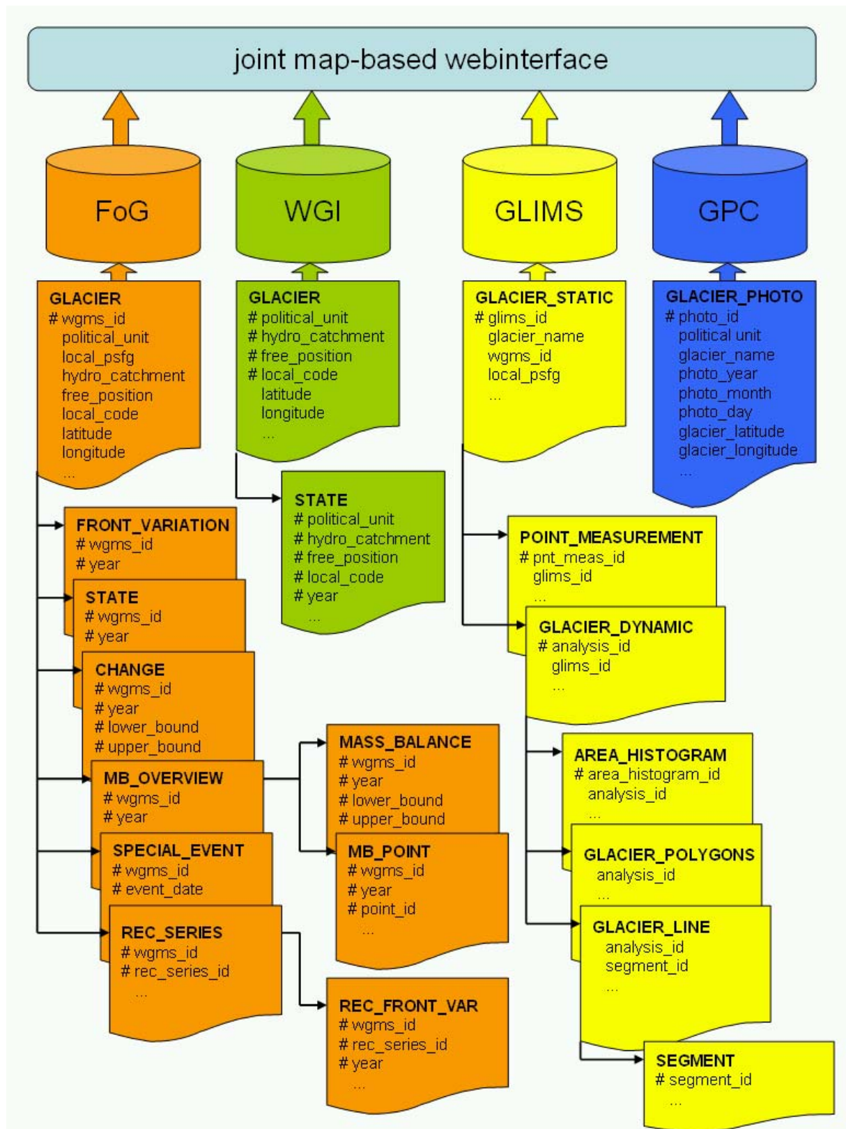
Figure 3.2: Schematic overview of the four glacier databases within the Global Terrestrial Network for Glaciers (GTN-G) storing Fluctuations of Glaciers (FoG), the World Glacier Inventory (WGI), the Global Land Ice Measurements from Space inventory (GLIMS), and the Glacier Photograph Collection (GPC). For all relational databases, the principal relations (upper-case letters) are shown with the attributes (lower-case letters) forming corresponding primary keys (#) and defining the glacier location.
