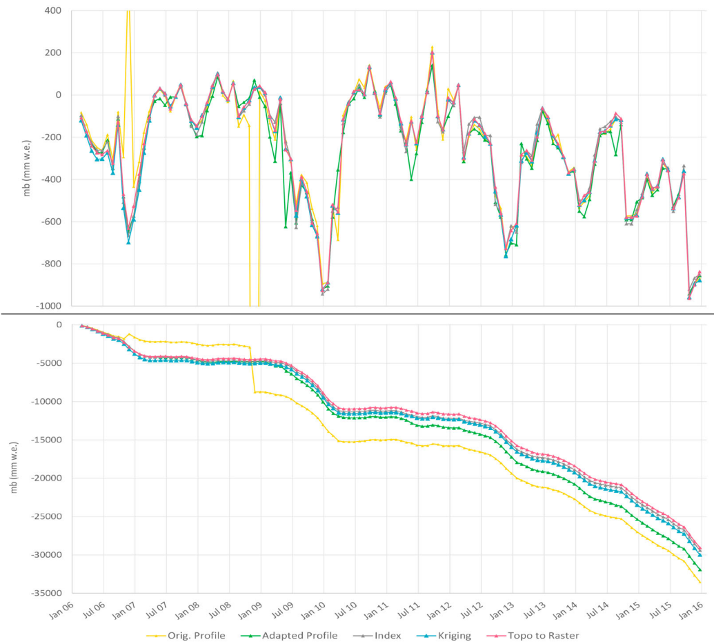
Figure 2. Comparison of monthly mass balance results from different interpolation methods. The inset table shows the final cumulative results for the full period.
