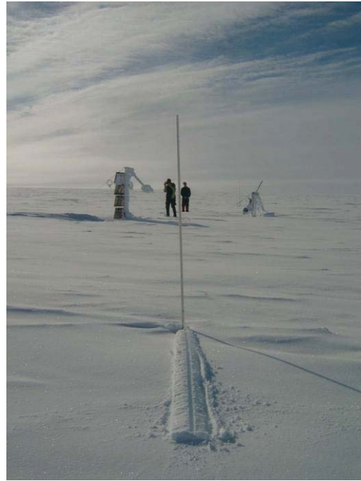
Figure 10. Rime, or possibly hoar , recently dislodged from an accumulation stake by solar heating (foreground) and still coating meteorological instruments (background), on Vestfonna, Svalbard.
